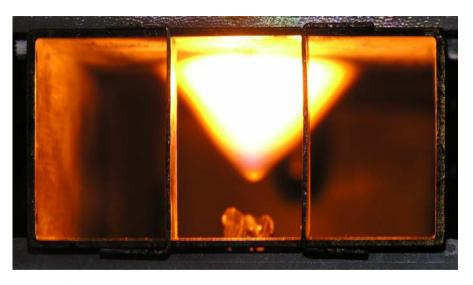
A fireball ejected from molten glass by localized microwaves
